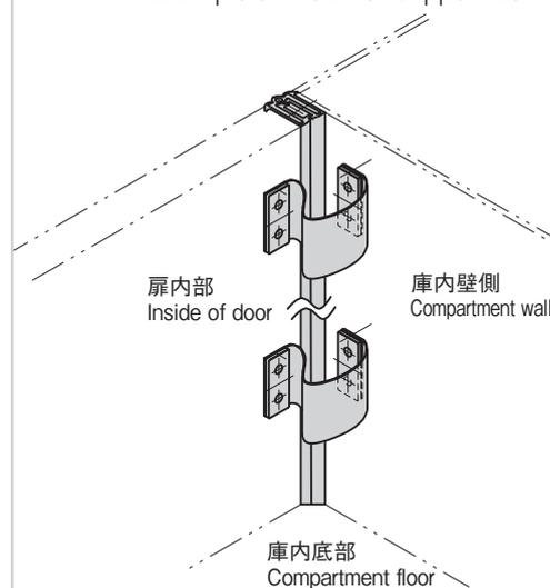
HINGES FOR SPECIALLY-EQUIPPED VEHICLES
